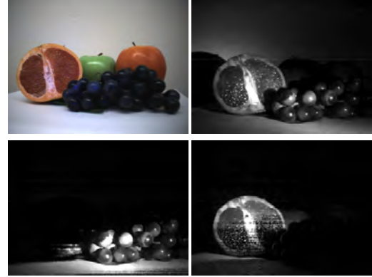
Figure 1. Row 1: Images of a scene captured with regular vision camera under ambient lighting (left) and a single-photon sensitive SPAD array under diffused laser illumination (right). Row 2: The temporal response approximately 703 ps (left) and 1171 ps (right) after emitting a pulse of light into the scene.
